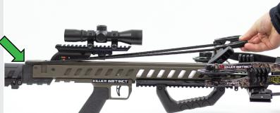
Pull rope cocker sled hook over the scope #3 and position on the crossbow string. Make sure rope is not hooked on any scope turrets and runs along the barrel.
