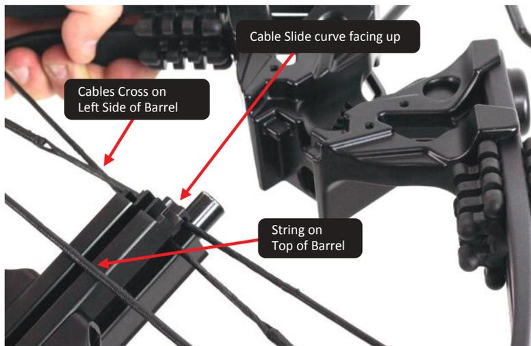
**CAREFULLY INSERT CABLES AND CABLE SLIDE INTO BARREL SLOT TO PREVENT CABLE PINCHING OR CABLE CONTACT WITH EDGES OF BARREL! CABLE SLIDE MUST BE INSTALLED BEFORE ATTACHING FRONT END!**
