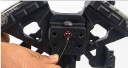
Insert foot stirrup (notches facing down) and align square notches with (2) set screw holes.
